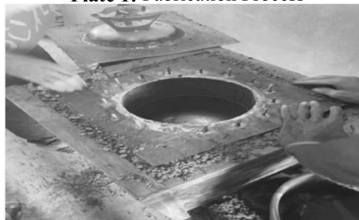
Plate 2: Process of Filling the Reactor by Lagging with Clay Soil
